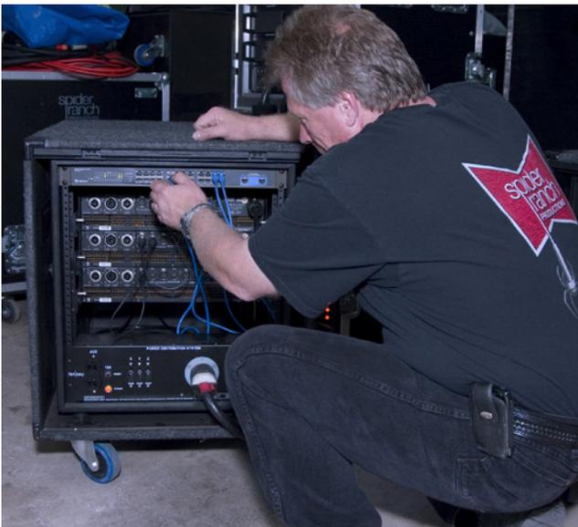
Alex Moran setting up the Lab.gruppen PLM amps an Ethernet cable connects the switch at the top of this amplifier stack to another switch at Front of House
