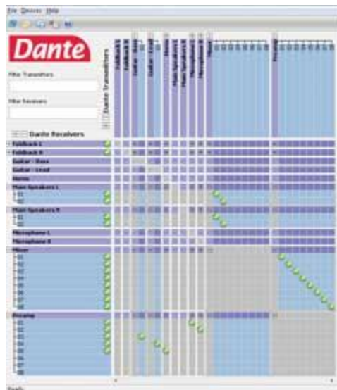
FIG. 1: Audinate's controller software provides matrix routing of all audio signals on the network. Photo: Courtesy Audinate
