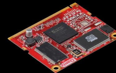
Audinate's Brooklyn provides all the core networking, control and monitoring functions needed for products such as DSP processors, amplifiers, digital snakes and break-in/break-out boxes, allowing manufacturers to more easily develop Dante-enabled products.
